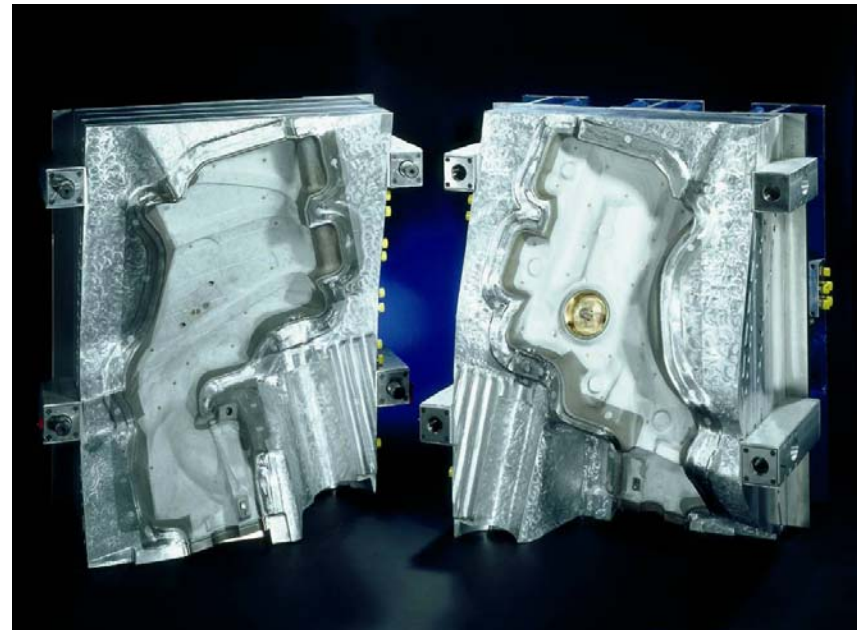
Moulds for a car fuel tank (Volkswagen)
